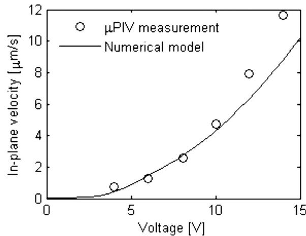
FIG. 4. Comparison between  $\mu\text{PIV}$  fluid velocity measurements and numerical simulation results as a function of voltage,  $V$ . The working volume is  $76 \mu\text{l}$  of de-ionized water and velocity is measured in the region of interest shown in Fig. 3(b) at  $z=400 \mu\text{m}$  from the well bottom.
